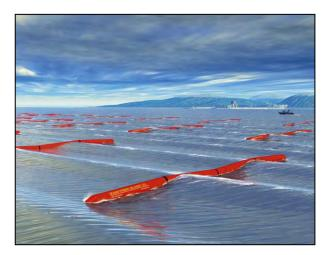
Visual simulation of wave energy attenuator devices. Image credit: US Dept. Of Energy
