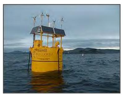
Point absorber buoy for capturing wave energy. Image credit: US Dept. of Energy
