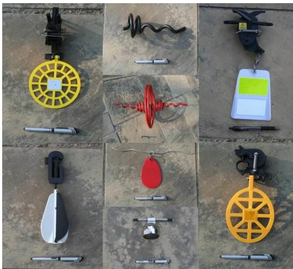
Figure 21: Various line marking devices (not comprehensive). In each photo a pen (circa 14 cm length) is placed to provide scale (Photo: EWT-WEP).
