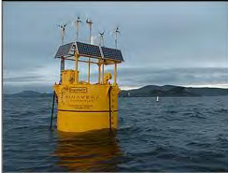
*Point absorber buoy for capturing wave energy.
